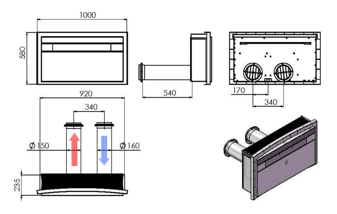
**Note:** The external pipes have two different diameters, use Ø160 mm for air inlet side and Ø150 mm for air out let side.
