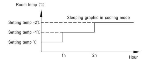
11.3.6.3 Under the heating mode, at the beginning of sleeping running, if environment temperature < setting temperature, the compressor, outdoor fan motor and indoor fan motor and four-way valve will be worked. If environment temperature ≥setting temperature, it will directly go into the sleeping mode running (see the below graphic). Fan speed will be fixed to be low speed. Wind direction can be adjusted or stay on one position.
